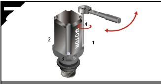
Tighten the mounting bolts in 1~4 order with approx 41Nm.
