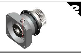
Rotate the set collar until the bolt hole is aligned with access hole.
