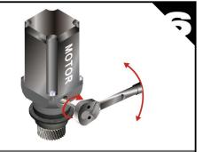
Set at vertical position. Tighten the mounting bolts (including washer) in 1~4 order with approx 2.1Nm.
